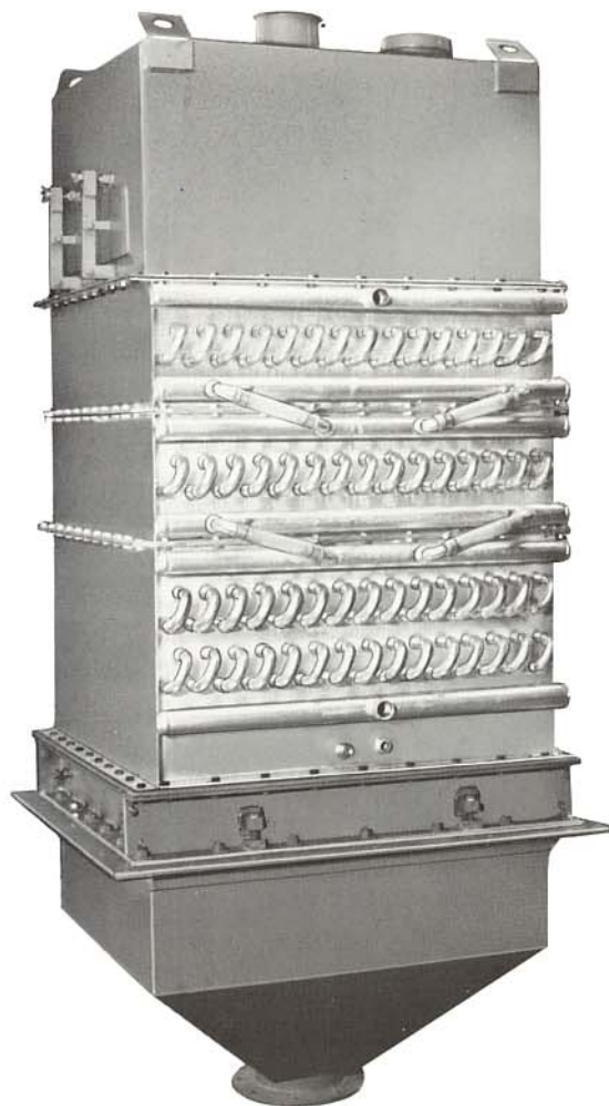
Completely installed reflux cooler
