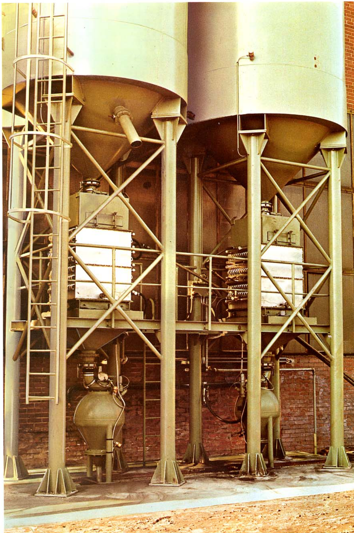
Application of 2 reflux coolers type KUE 199 below 2 silos for used sand
